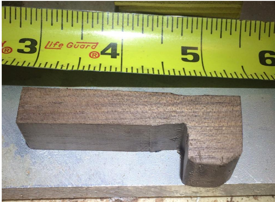
Photo 6. A walnut “shoe”. It is important that the heel is a little taller than the thickness of the wood that the parts are being made from. This piece should be made from hardwood.
