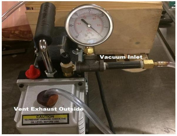
The 2.5 cfm vacuum pump from Harbor Freight works well, but you should modify the exhaust by making a tapered plug to fit the hole and pipe the exhaust outside to avoid breathing the oil mist. The pump will slowly lose oil as the mist condenses inside the tube and makes its way out. Yes, a better solution is needed.
